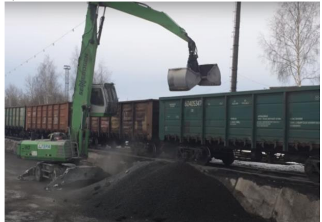
Fig. 2. Unloading open wagons with grab buckets: a) in seaport conditions, b) in the conditions of a private enterprise
