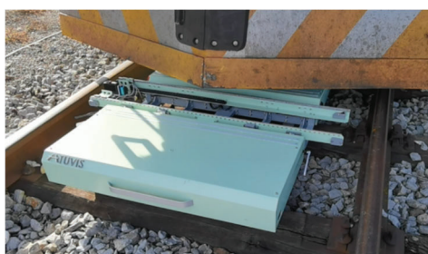
Fig. 13 ATUVIS positioned on the track, below the train
