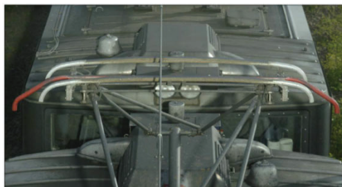
Fig. 11 Pantograph monitoring system [16]
