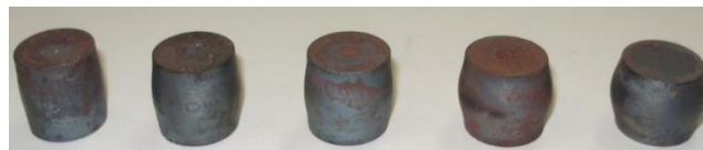
Fig. 6. Samples after tests performed at various reductions
