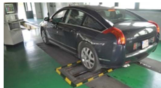
Figure 3. Passenger vehicle in the rolling brake test room
