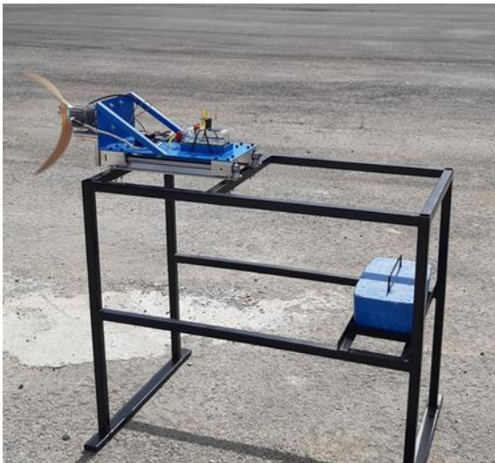
Figure 22: Engine run-in DLA 64. Source: Authors
