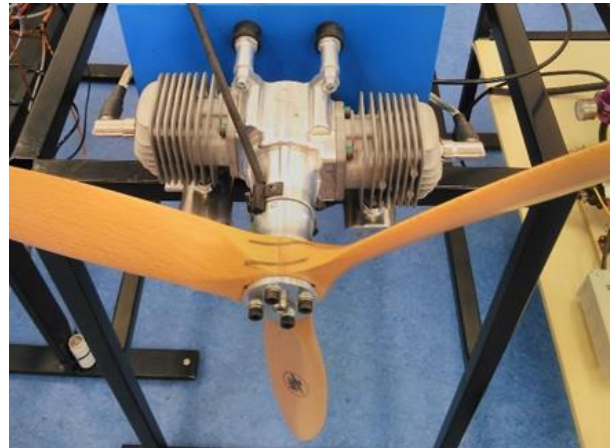
Figure 21: Internal combustion engine DLA 64 with three-bladed propeller. Source: Authors.
