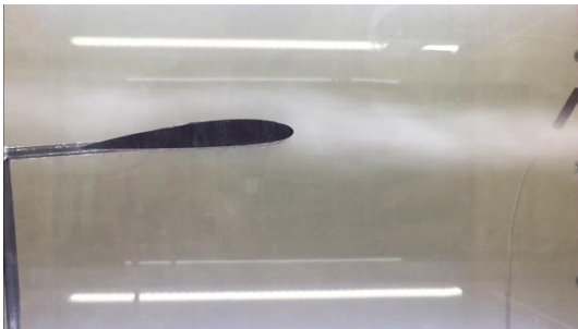
Figure 9: Air flow visualisation after the installation of honeycomb screen. Source: Authors.
