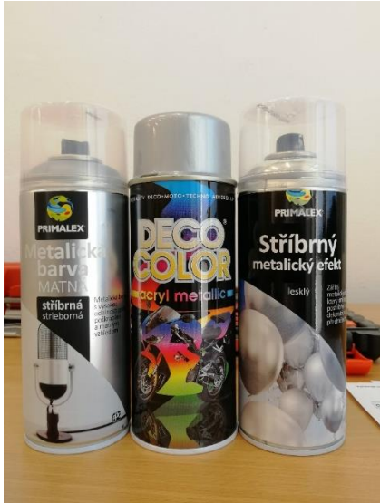
Figure 3: Upper metallic coatings sprays. Source: Authors.
