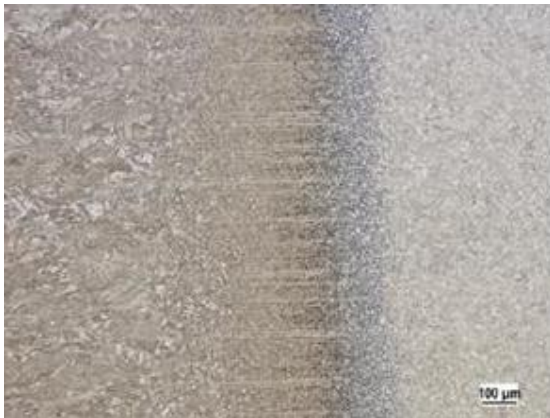
Fig. 2. Transfer of the metal being welded into the area affected by the heat of the material Strenx 960 using the electron beam technology
