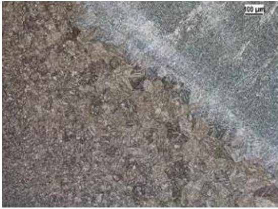
Fig. 1. Microstructure of the basic material Strenx 960 , transfer of the metal being welded to the area affected by the heat using the MAG technology
