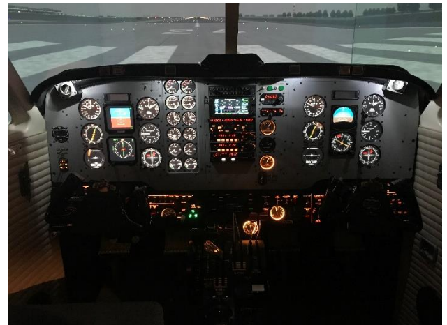
Figure 1: Cockpit ergonomics of the flight simulator in Beechcraft King Air B200 (Generic). Source: Autor.
