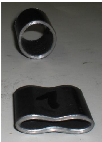
Fig. 9. Test sample before and after technological compression test
