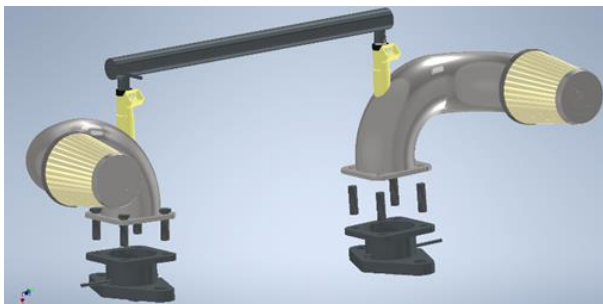
Figure 7: Modification of the original design associated with a 180° rotation of the intake manifold [author]
