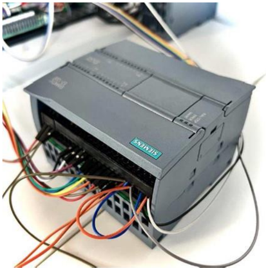
Fig. 2. PLC Simatic S7-1200
