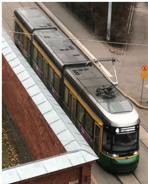
Fig. 4 Fully covered roof area of ForCity Smart ArtOc X34 LRV in Helsinki
