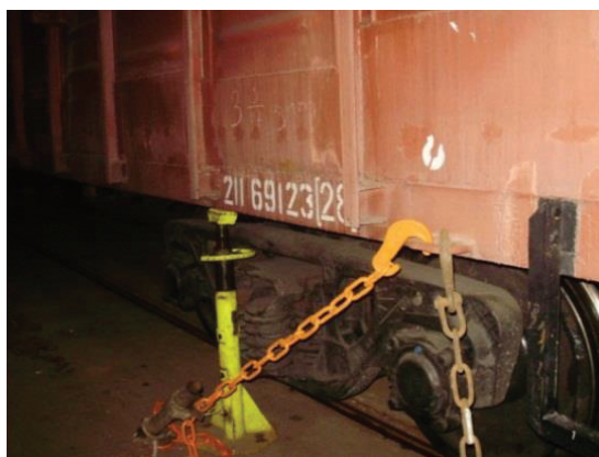
Fig. 2 Scheme of fixing the covered wagon on the deck of the railway ferry
