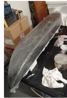
Figure 23 - Laminated part of UAV hull
