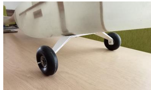
Figure 31 -Main gear mounted on UAV fuselage
