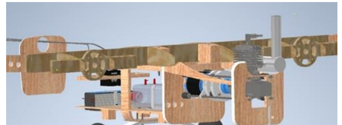
Figure 6 - AutoCAD INVENTOR fuselage wooden inner construction
