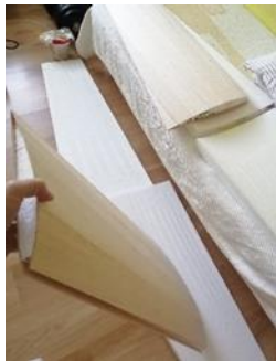
Figure 19 -Applied wing balsa cover
