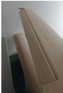
Figure 20 -Mounted aileron on tapered wing part
