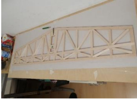
Figure 26 - Horizontal stab with elevator assembly
