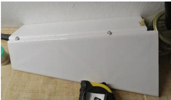
Figure 28 - Done vertical tail surface
