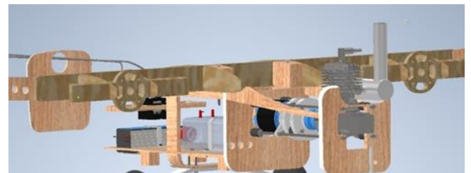
Figure 6 - AutoCAD INVENTOR fuselage wooden inner construction
