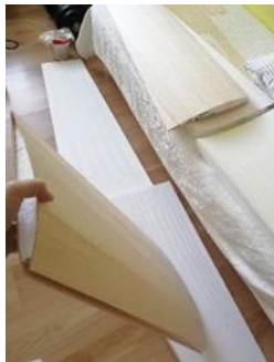
Figure 19 -Applied wing balsa cover
