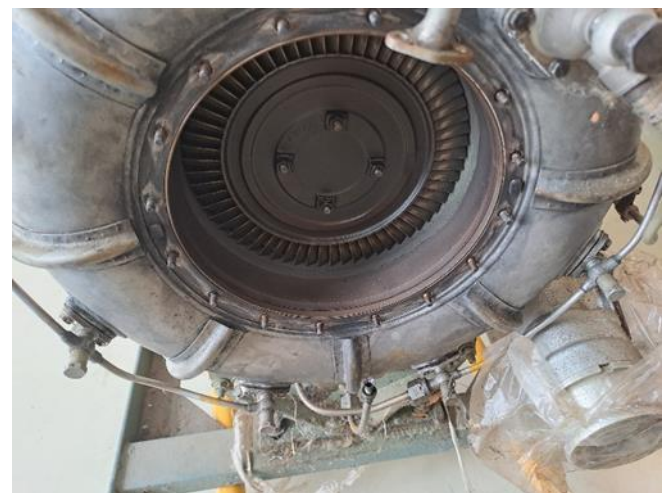
Figure 4 - Exposed power turbine of the AI-9 engine
