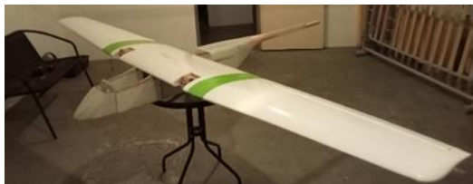
Figure 21 -Done UAV wing
