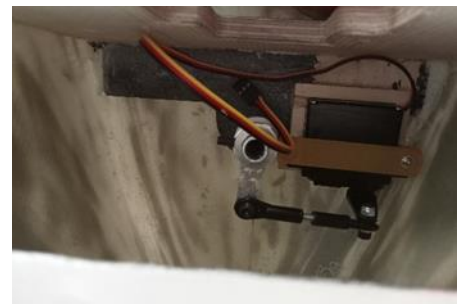
Figure 32 - Front gear servo engine ride system mounted on UAV
