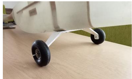
Figure 31 - Main gear mounted on UAV fuselage
