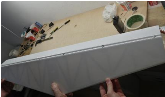
Figure 27 - Done horizontal tail surface
