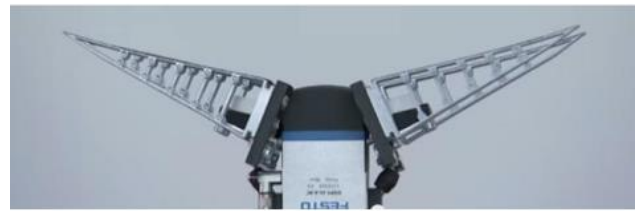
Fig. 1. The bionic adaptive gripper [1]
