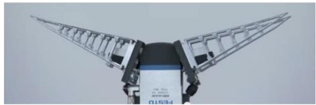
Fig. 1. The bionic adaptive gripper [1]
