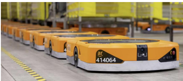
Fig. 2. Amazon Robotics' GTP warehouse robots [4]
