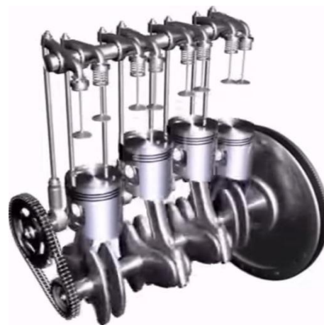
Fig. 1. An example of the OHV valvetrain [1]
