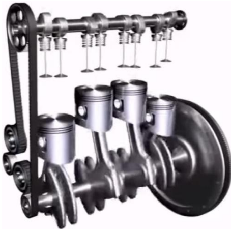
Fig. 3. An example of the SOHC valvetrain [1]
