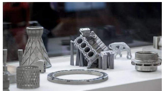
Fig. 6. Printed metal parts [9]
