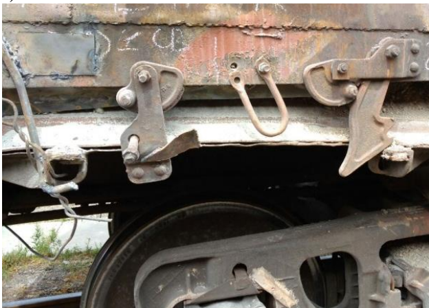
Fig. 1. Damage of hatch covers of open wagons: a) deformation, b) damage of the cast
