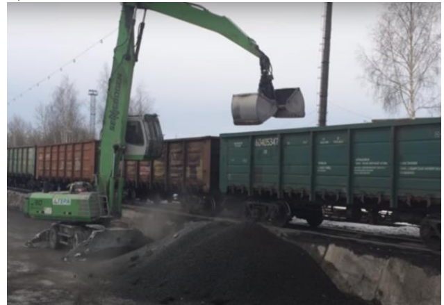
Fig. 2. Unloading open wagons with grab buckets: a) in seaport conditions, b) in the conditions of a private enterprise
