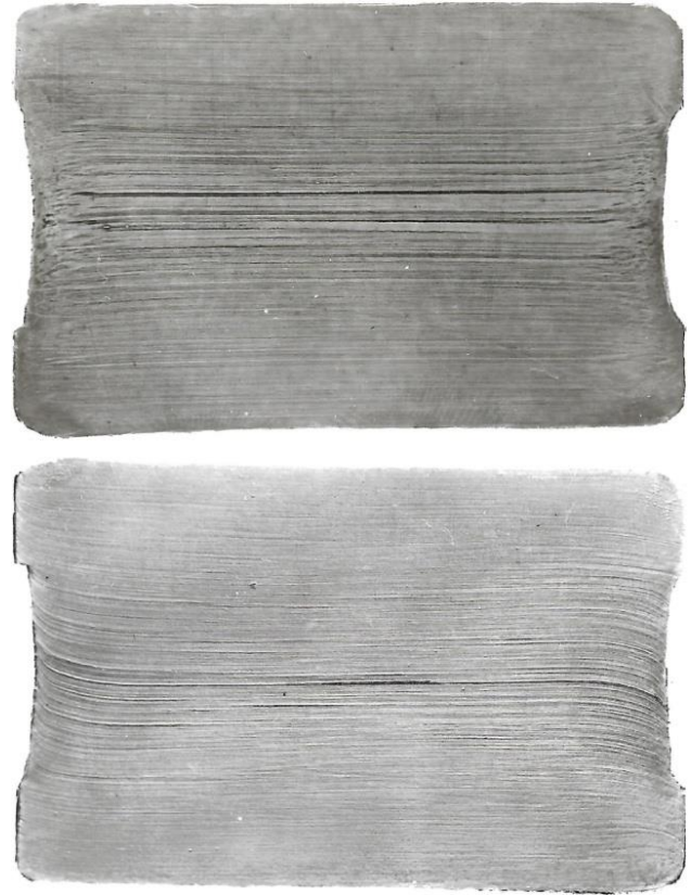
Fig. 7. The course of compressed fibre after forming
