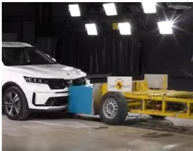
Obr. 72 Moving Progressive Deformable Barrier (MPDB) [45] [46]
