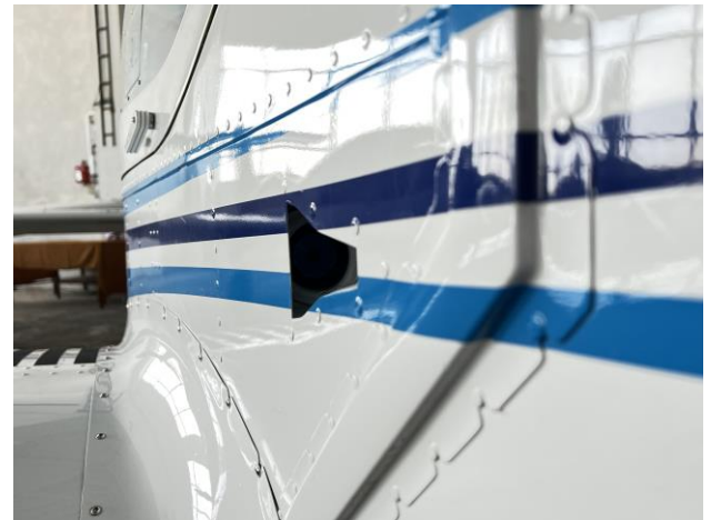
Figure 5: Sensor's installation in air intake. Source: Authors
