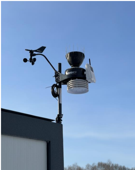
Figure 6: Weather station Davis Instruments Vantage Pro2 instalment. Source: Authors.
