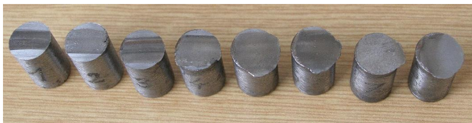
Obr. 4 Rozvoj degradace kontaktn  plochy s dobou zatěřov n  Fig. 4 Development of contact surface degradation with loading time
