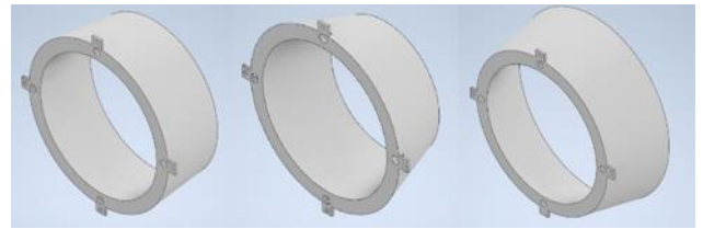
Figure 3 Constant, convergent and divergent shape of nozzle
