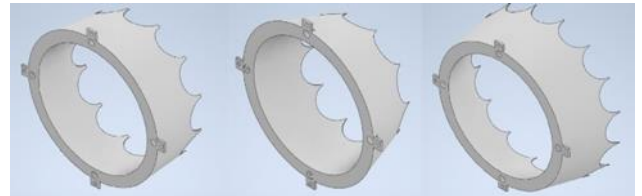
Figure 4 Constant, convergent and divergent shape of nozzle with special shaped edge
