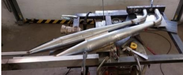
Figure 7: Exhaust system production. [Source: Authors]
