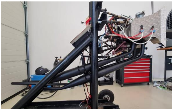
Figure 8: Exhaust system installation. [Source: Authors]
