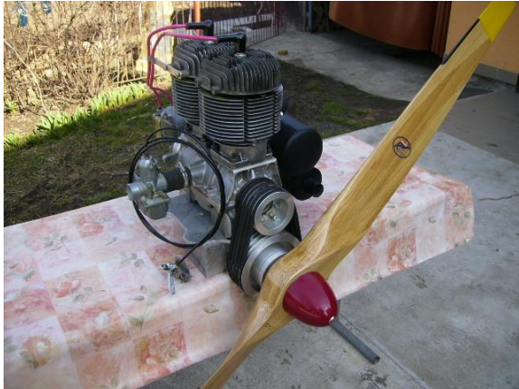
Figure 6: Engine for ultralight aircraft. [authors]
