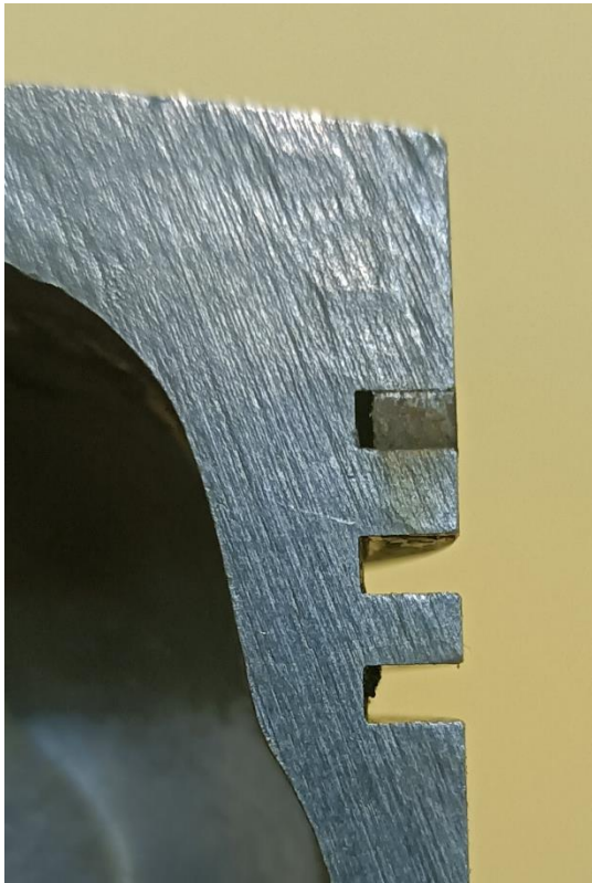
Figure 1. A cut of the piston together with the piston ring, engine P65, we would like to draw attention to the minimum distance between the piston ring and the upper edge of the groove
