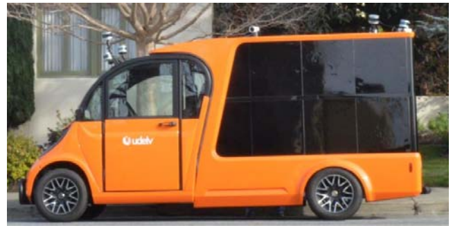
Figure 2. Autonomous Ground Vehicles with Lockers
