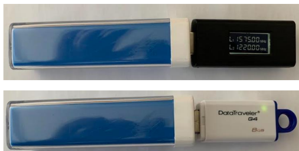
Figure 2: GPS jammer from e-shop. Source: Authors.
