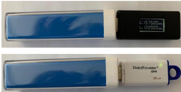
Figure 2: GPS jammer from e-shop. Source: Authors.
