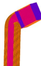
Figure 10: Detail of the numerical simulation of the steel column collapse with additional ribbing (left) and additional ribs on steel H-profile building structure beam (right). Source: Authors.
