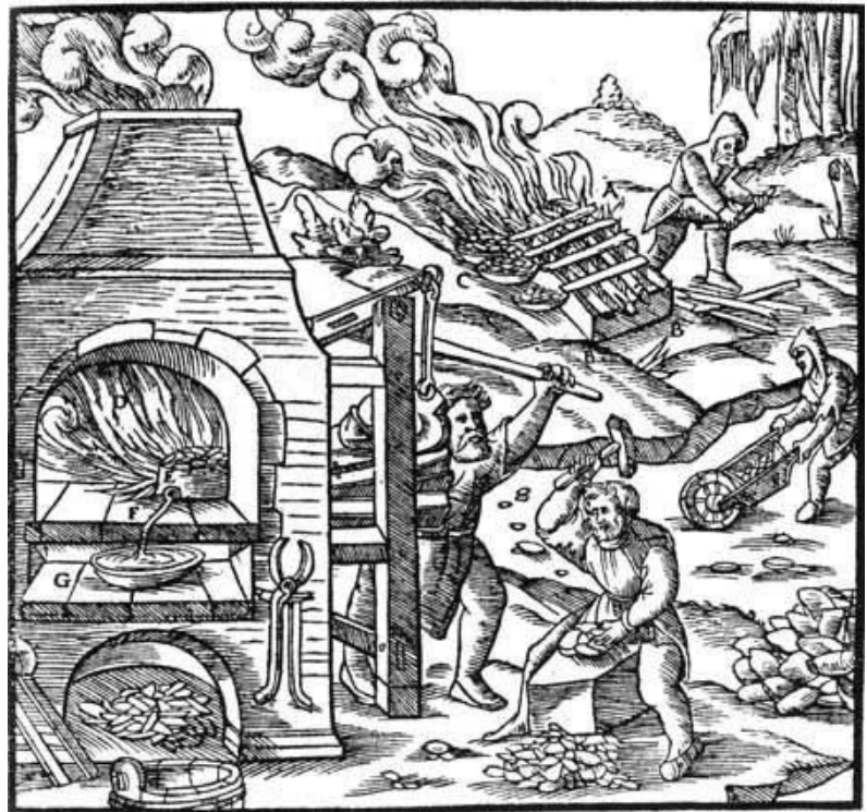
A—WOOD. B—BRICKS. C—PANS. D—FURNACE. E—CRUCIBLE. F—PIPE. G—DIPPING-POT.
