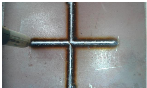
Fig. 5. The first layer welding of variant No. 3
