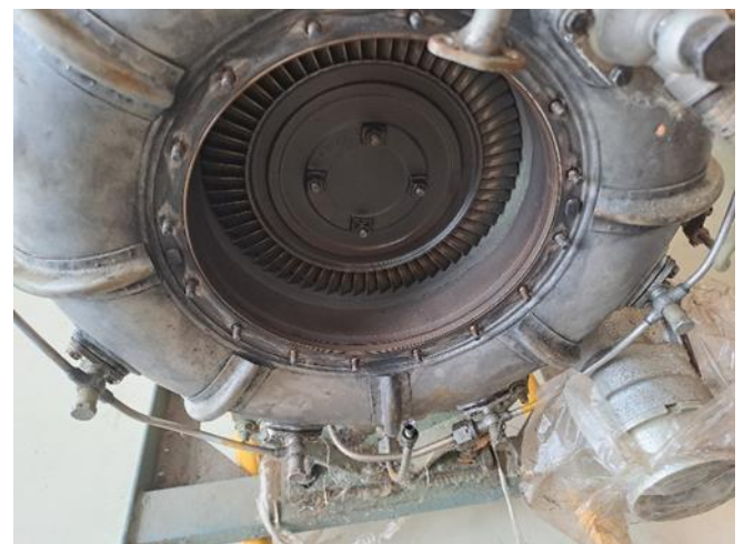
Figure 4 - Exposed power turbine of the AI-9 engine
